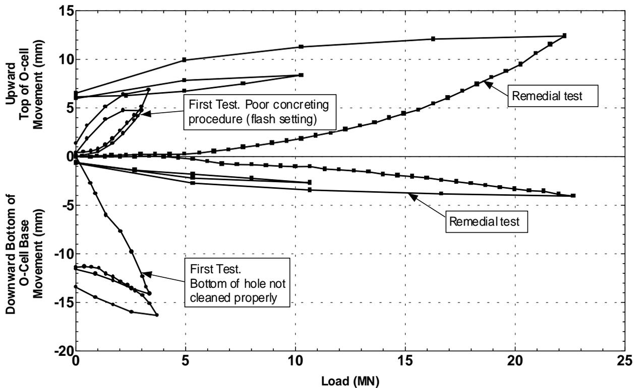
**Fig. 8 - Example 723, effect of poor cleanout procedures in weathered rock (EB) and effect of poor concreting procedures (SS)**
