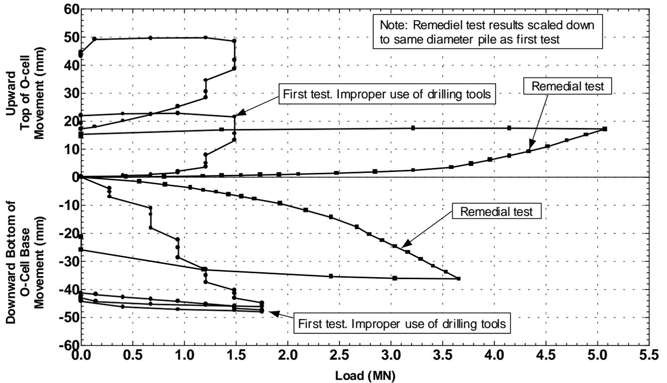
**Fig. 6 - Example 562, improper use of drilling tools**
