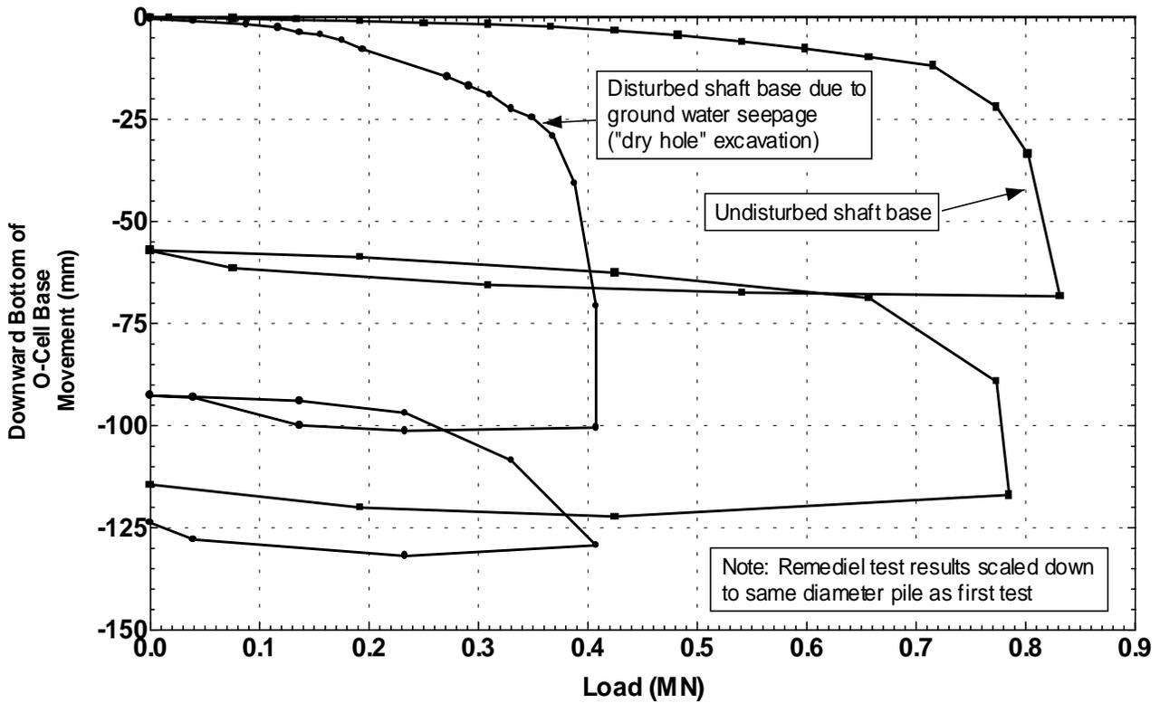
**Fig. 7 - Example 643, effect of poor cleanout procedures ("dry hole") in clay**
