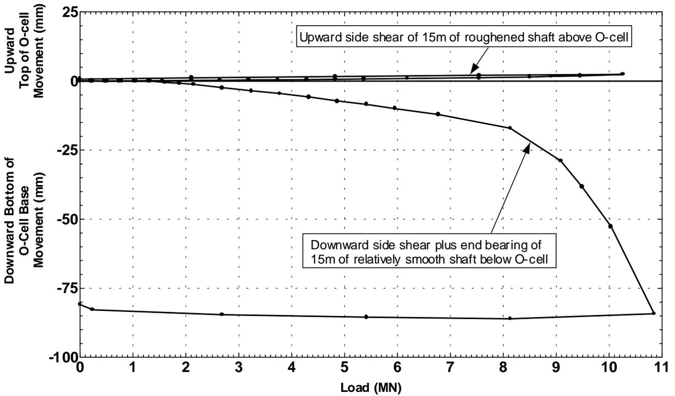
**Fig. 5 - Example 561, effect of wall roughening**
